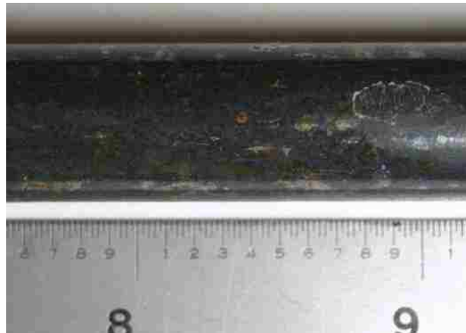
Figure 4.13: A typical representation of the surface condition along a smooth pure enamel-coated specimen after the salt spray test.
