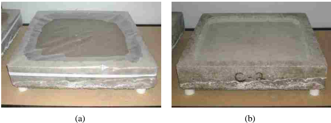
Figure 3.5: Typical ponding specimen during either the wet or dry phase of testing. (a) Wet phase. (b) Dry phase.
