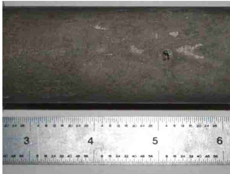
Figure 5.5: A void considered to be detrimental to the grouted specimen's performance in the ACT test.
