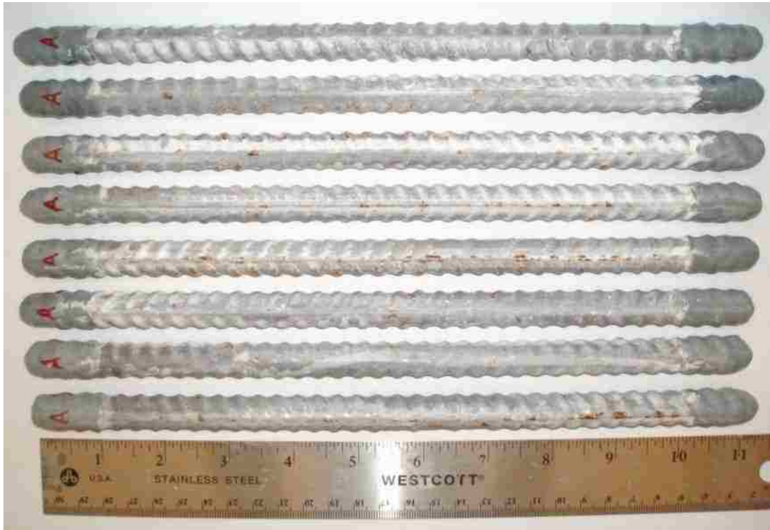
Figure B - 6: Right side of the deformed 50/50 enamel-coated salt spray specimens after testing.
