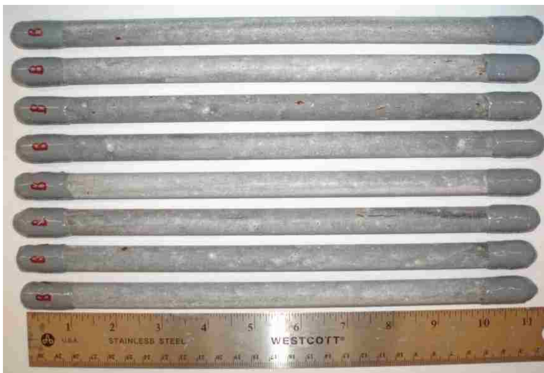
Figure B - 9: Backside of the smooth double enamel-coated salt spray specimens after testing.
