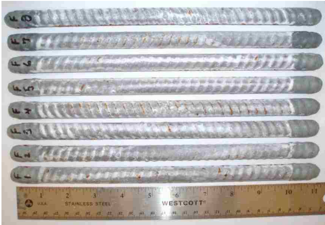
Figure B - 4: Front side of the deformed 50/50 enamel-coated salt spray specimens after testing.
