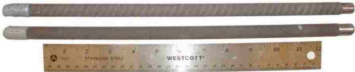
Figure 5.1: A typical smooth and deformed coated bar prepared for the ACT method.
