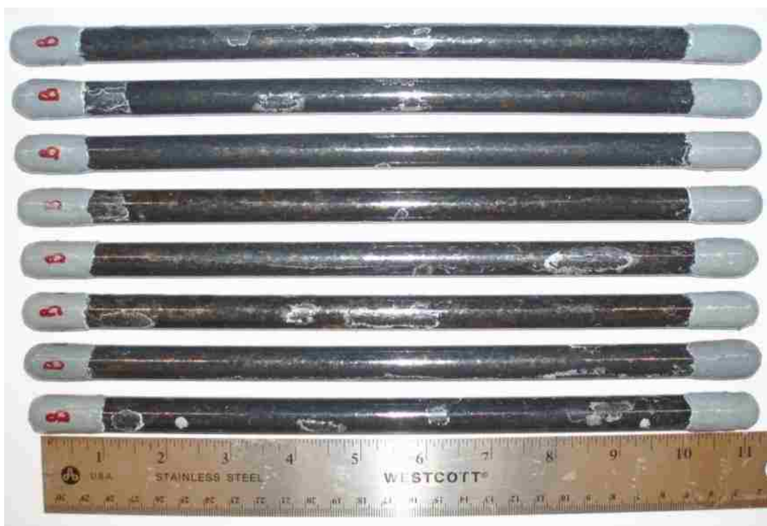
Figure B - 15: Backside of the smooth pure enamel-coated salt spray specimens after testing.
