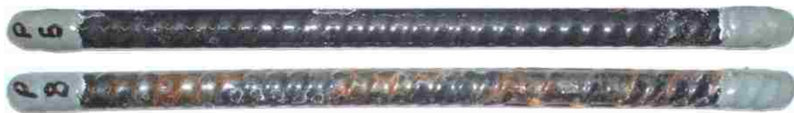
Figure 4.11: A visual comparison between a deformed pure enamel-coated specimen that performed well and one that performed poorly.
