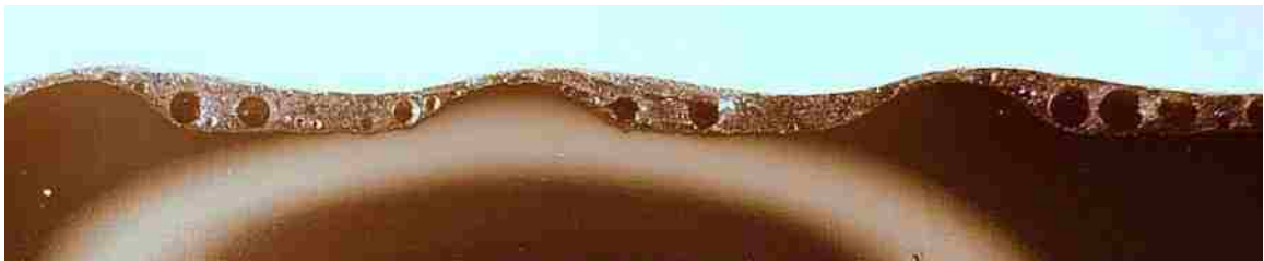
Figure 4.14: Cross-sectional views of the pure enamel coating along smooth and deformed specimens. (a) A longitudinal view of the pure enamel coating distributed along a deformed specimen that had performed well during the test.
