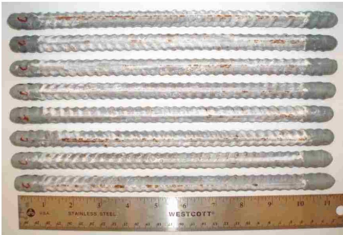
Figure B - 7: Left side of the deformed 50/50 enamel-coated salt spray specimens after testing.
