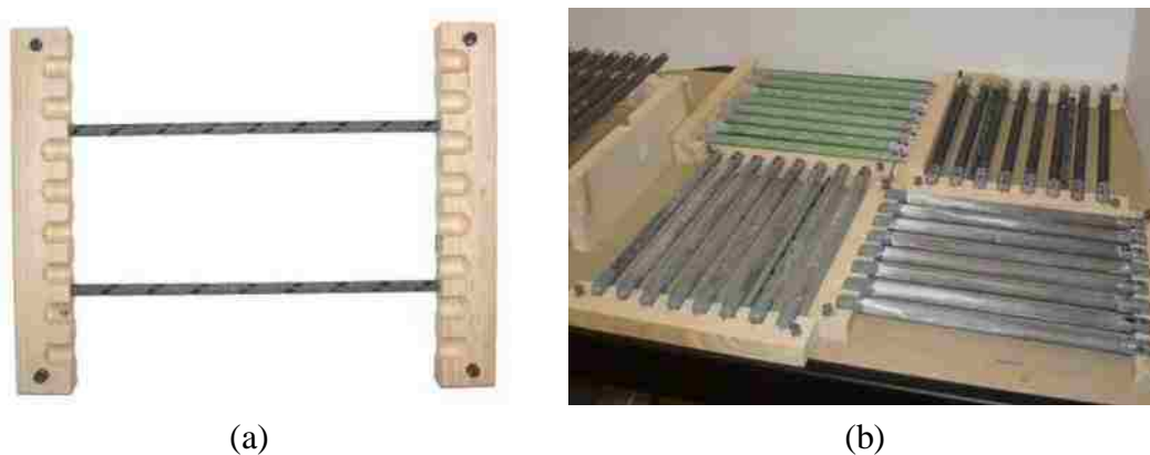
Figure 4.4: Specimen layout during the dry phase of testing. (a) Rack used to support a set of salt spray specimens. (b) Overall layout.
