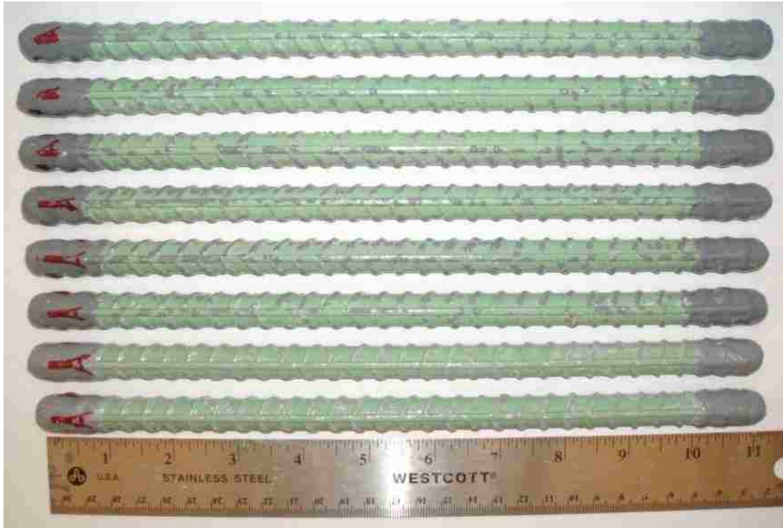
Figure B - 24: Right side of the deformed epoxy-coated salt spray specimens after testing.
