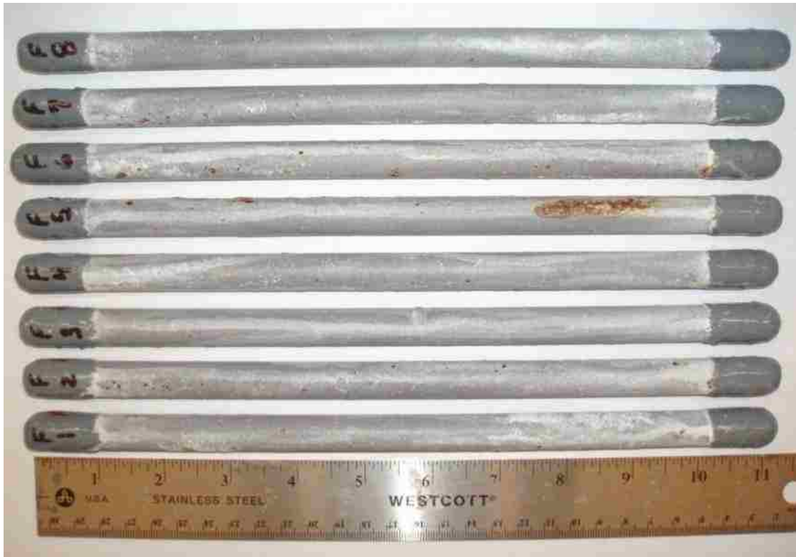
Figure B - 2: Front side of the smooth 50/50 enamel-coated salt spray specimens after testing.
