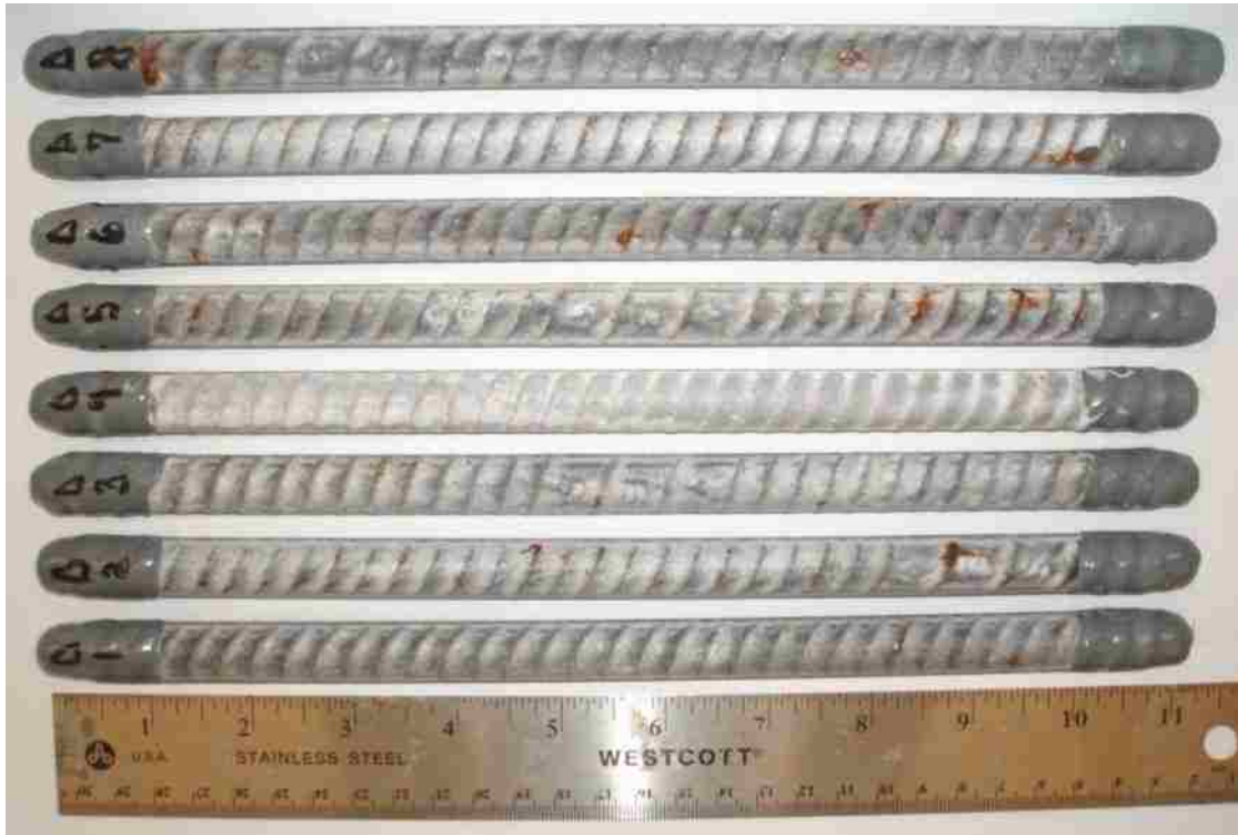
Figure B - 10: Front side of the deformed double enamel-coated salt spray specimens after testing.
