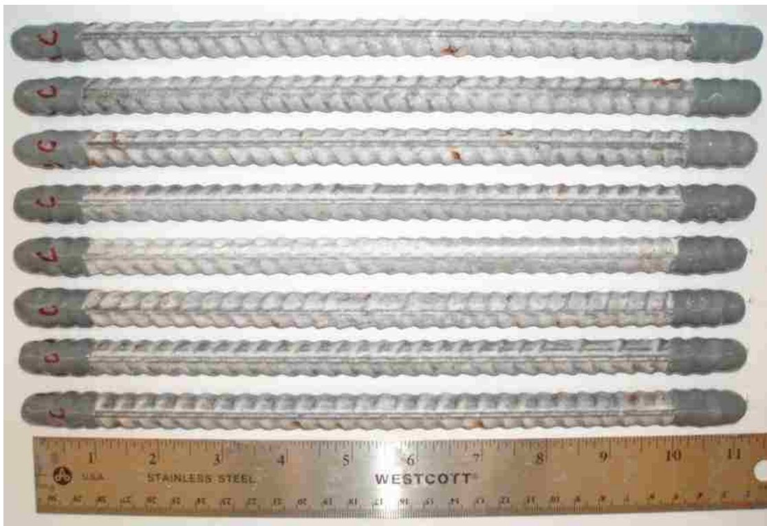
Figure B - 13: Left side of the deformed double enamel-coated salt spray specimens after testing.
