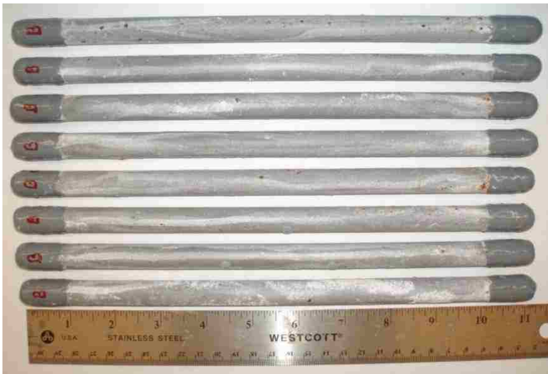
Figure B - 3: Backside of the smooth 50/50 enamel-coated salt spray specimens after testing.
