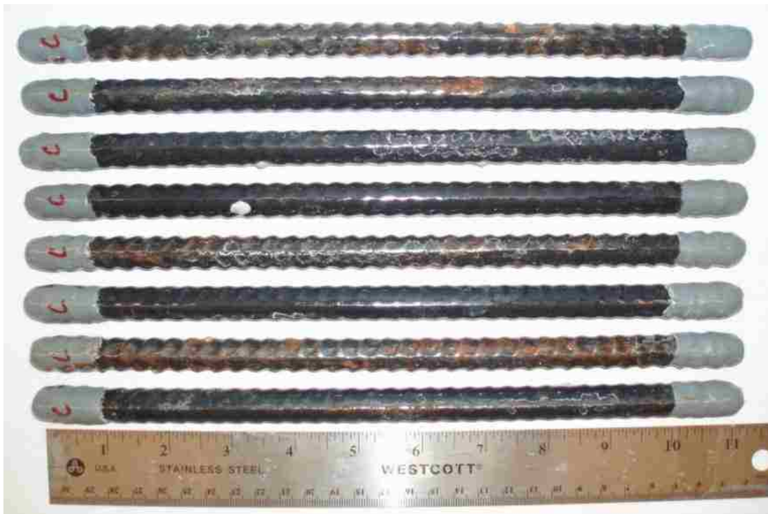
Figure B - 19: Left side of the deformed pure enamel-coated salt spray specimens after testing.
