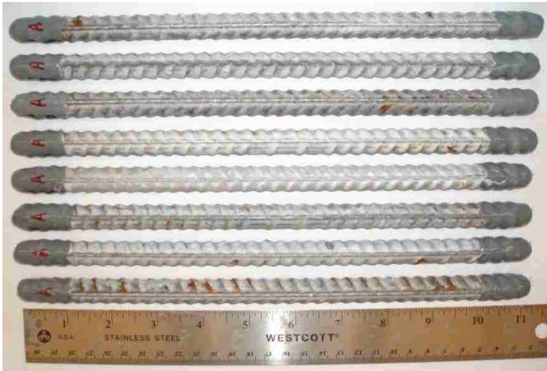
Figure B - 12: Right side of the deformed double enamel-coated salt spray specimens after testing.
