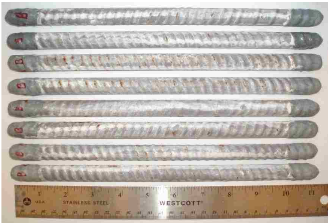
Figure B - 5: Backside of the deformed 50/50 enamel-coated salt spray specimens after testing.
