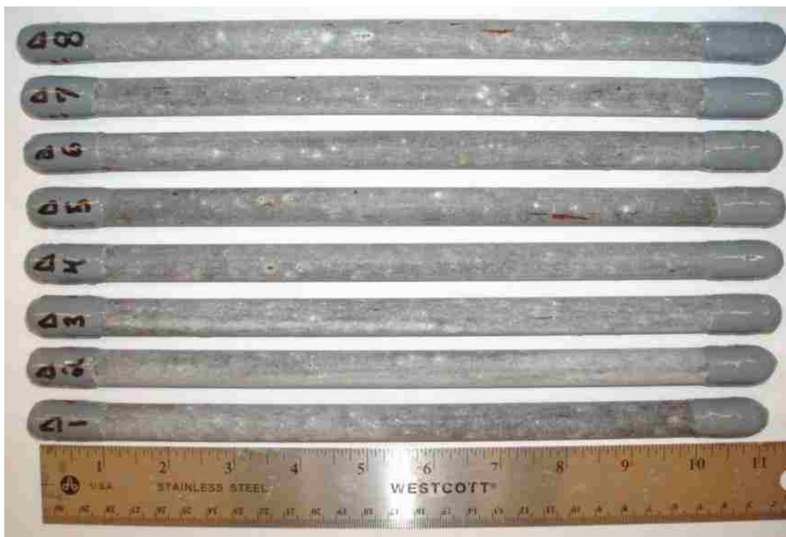
Figure B - 8: Front side of the smooth double enamel-coated salt spray specimens after testing.
