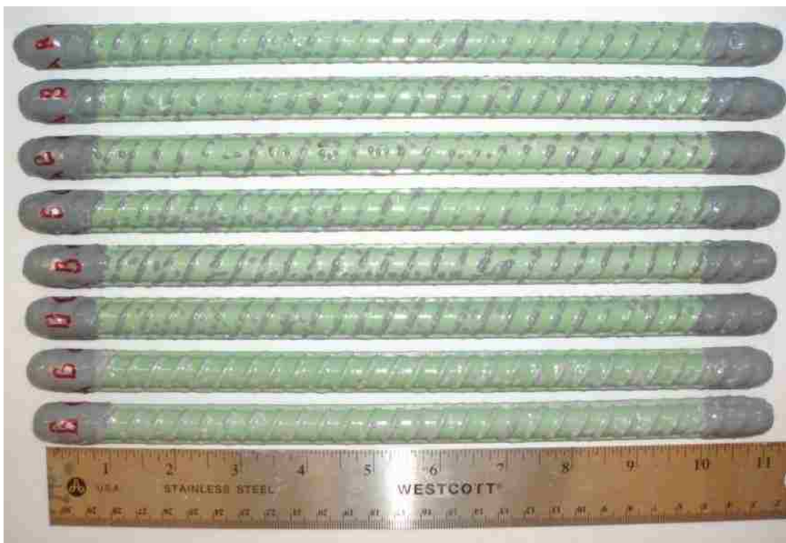
Figure B - 23: Backside of the deformed epoxy-coated salt spray specimens after testing.
